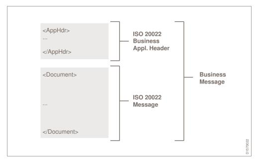
The Business Application Header is available as an additional XML schema, which comes on top of the business payload. It replaces the application header that is found today in some of the MX messages. New ISO 20022 messages and new versions of existing MX messages will progressively require the Business Application Header.
