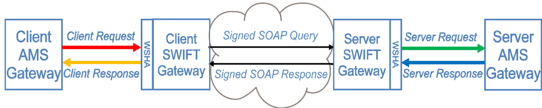
Figure 6: The Web Services Host Adapter on the SWIFT Gateway consolidates multiple SOAP messages into a single, synchronous request-reply interaction
